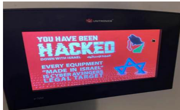
HMI defacement by CyberAv3ngers using default password `1111`
